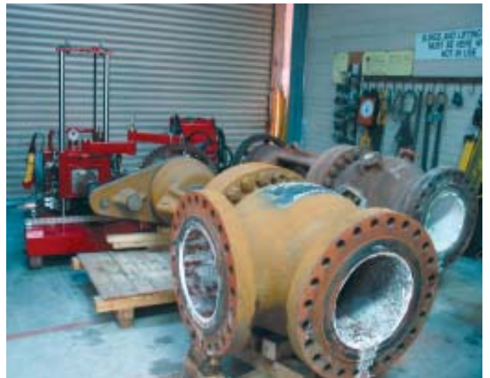
The valve grinding unit undergoing workshop trials.
